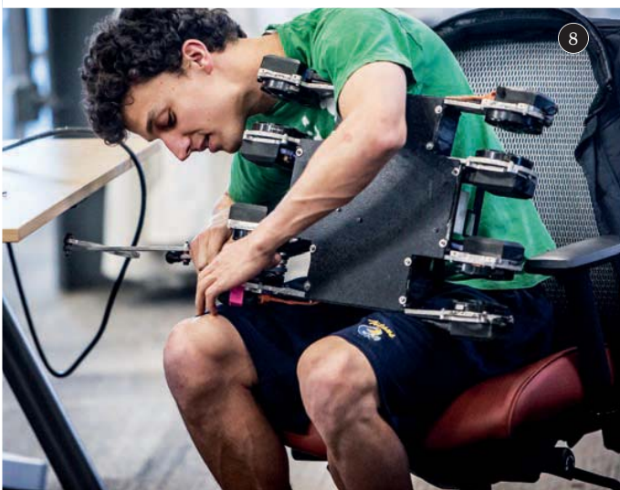
6. The Cyber Café offers snacks, drinks and a chance to connect with friends. 7. Researchers fabricate biosensors in the Singh Center for Nanotechnology. 8. Turner Topping, doctoral student in the Kod*lab at PERCH, attaches legs to the Minitaur robot. 9. Graduate student Emily Tess performs cell culture in the Huh lab. 10. Senior Lecturer Bruce Kothmann confers with students on a simulation model of a smart highway system in the Forman Active Learning Classroom.
